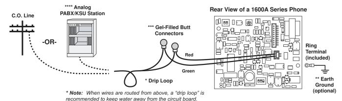
\*\*\* **Note:** The gel-filled (water-tight) butt connectors are designed for insulation displacement on 19-26 guage wire with a maximum insulation of 0.082 inches. Cut off bare wire ends prior to terminating.
